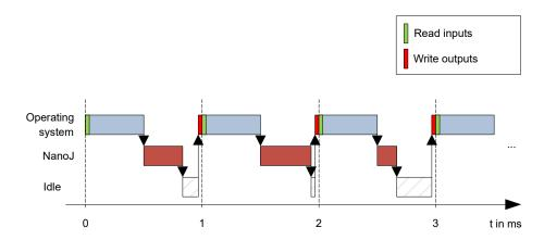
If the *NanoJ program* needs more time than was allotted, it is ended and an error code set in the object dictionary.
