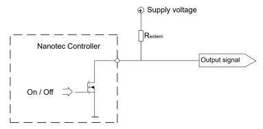
With a supply voltage of +24 V, a resistance value  $R_{\text{external}}$  of 10  $k\Omega$  is recommended.
