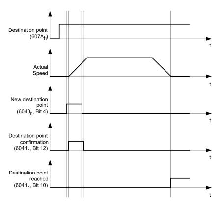
The controller can also reset bit 4 in object  $\underline{6040}_h$  (controlword) on its own. This is set with bits 4 and 5 of object  $\underline{60F2}_h$ .
