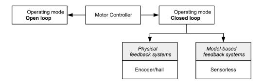
Summarized in the following are all possible combinations of control modes and feedback systems with respect to the motor technology. Support of the respective control mode and feedback is controller-specific and is described in chapters and Operating modes.
