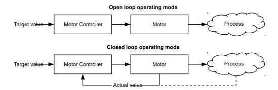
In addition to the physical feedback systems (e.g., via encoders or Hall sensors), model-based feedback systems, collectively referred to as sensorless systems, are also used. Both feedback systems can also be used in combination to further improve the control quality.
