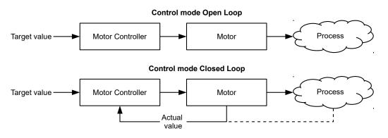
In addition to the physical feedback systems (e.g., via encoders or Hall sensors), model-based feedback systems, collectively referred to as sensorless systems, are also used. Both feedback systems can also be used in combination to further improve the control quality.
