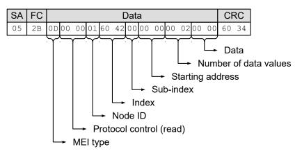
Shown as an additional example below, a sequence of Modbus messages is sent from the master to the slave to rotate the motor in "Velocity" mode:
