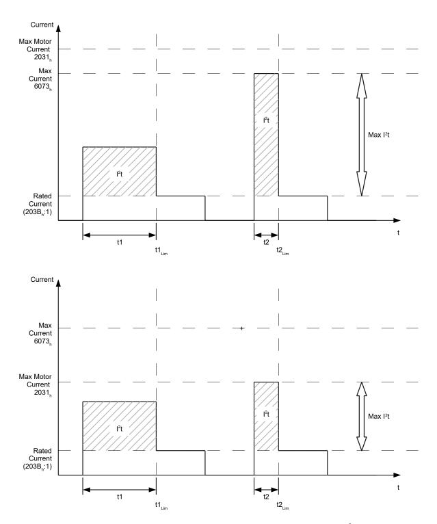
In the first section, t1, the current value is higher than the rated current. At time  $t1_{Lim}$ ,  $I^2 t_{Lim}$  is reached and the current is limited to the rated current. A current that corresponds to the maximum current then occurs for a period of time t2. Hence, the value for  $I^2 t_{Lim}$  is reached more quickly than in time t1.
