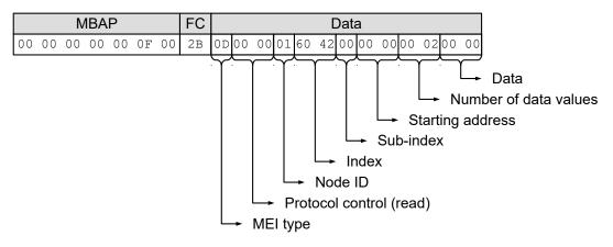
Shown as an additional example below, a sequence of Modbus messages is sent from the master to the slave to rotate the motor in "Velocity" mode:
