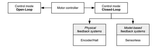
Summarized in the following are all possible combinations of control modes and feedback systems with respect to the motor technology. Support of the respective control mode and feedback is controller-specific and is described in chapters *Pin assignment* and **Operating modes**.
