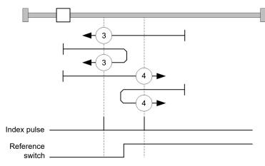
With methods 5 and 6, the right switching edge of the home switch is used as reference:
