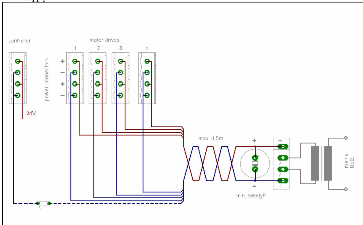
To reduce fault influences it is highly recommended to have separated power lines for each power drive. To avoid static charges when controller and power drive operates with different power supplies, it is a good praxis to insert a resistor of approx. 100kOhm between controller and power drive.
