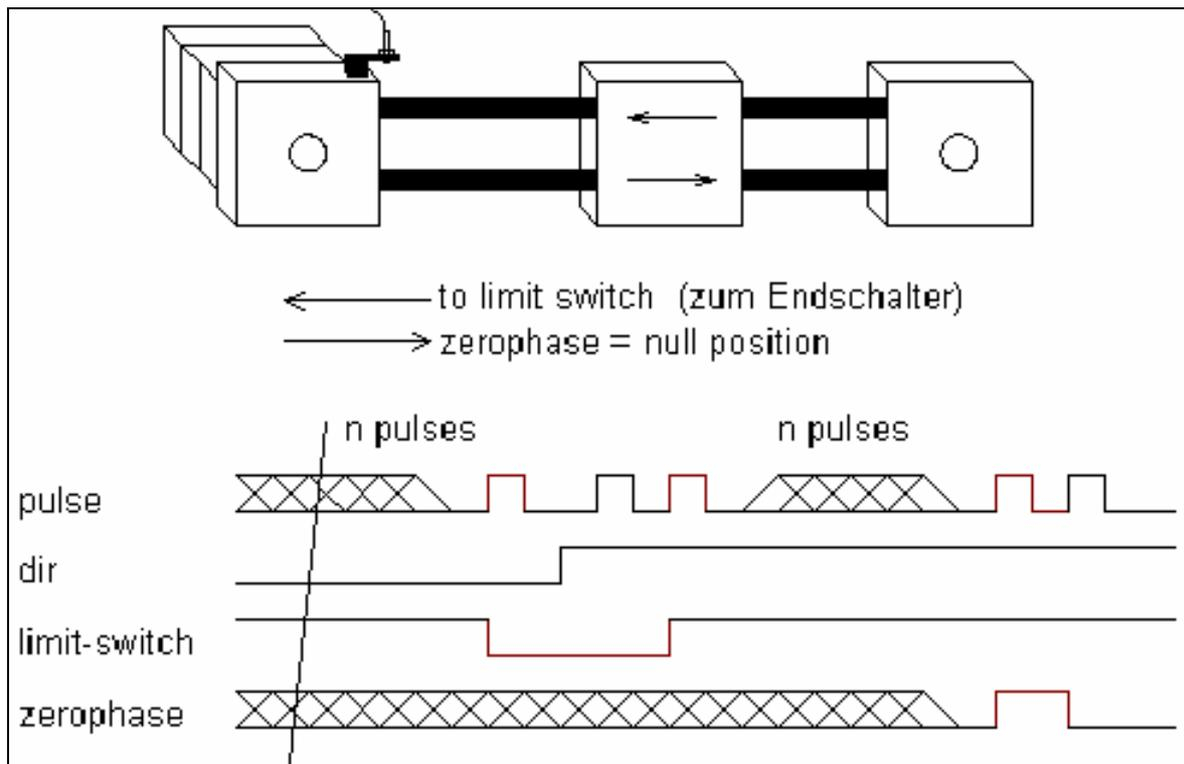
ZERO phase or ZERO position can be used as an exact reference point. Following is a procedure to handle with ZERO points.
