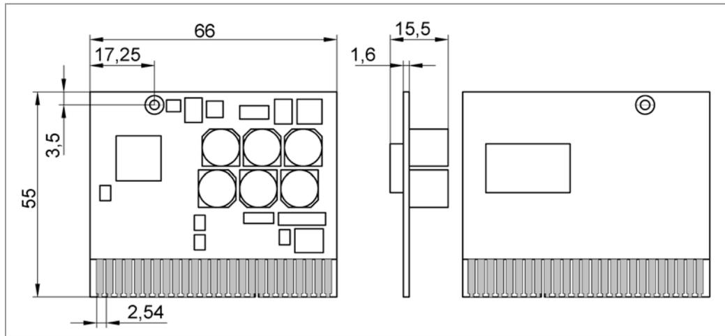
**SMCP33-K dimensions (with heat sink)**
