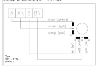
current per winding x 0,7 = current per Phase example: current / winding 1A = 0,7A / Phase
