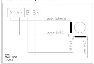
current per winding = current per Phase example: current / winding 1A = 1A / Phase
