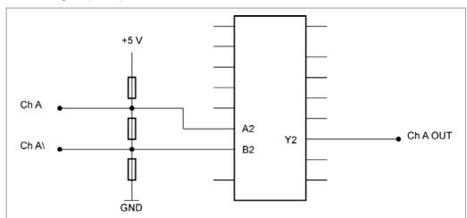
The SMCP controllers themselves currently cannot evaluate the differential signal, meaning that only the channels A, B and I need to be connected to perform position monitoring. We recommend shielding and twisting the encoder line to minimize interference with the encoder signal from the outside.
