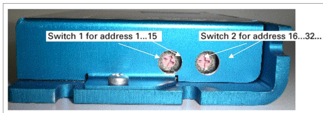
The 1st digit is set with switch 1 (left), the 16th digit of the address is set with switch 2 (right).
