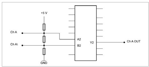
The SMCP controllers themselves currently cannot evaluate the differential signal, meaning that only the channels A, B and I need to be connected to perform position monitoring. We recommend shielding and twisting the encoder line to minimize interference with the encoder signal from the outside.
