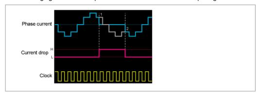
The grey lines in the figure show that the output stage has internally moved the motor four additional steps from position 1 to position 2. When the enable signal is reactivated (level on "Low"), motor operation continues from position 2 (only if the supply voltage  $V_{BB}$  remains in tact and the clock frequency is constant).
