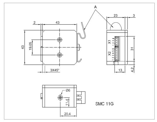
A: Retaining clip for DIN rail
