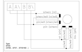
8 lead wire - serial for low frequency < 1 kHz
