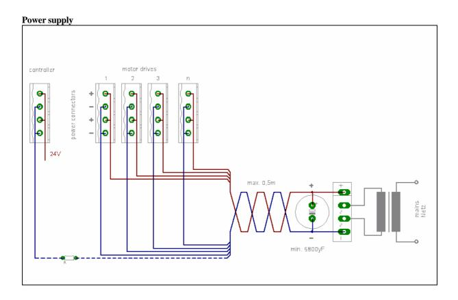
To reduce fault influences it is highly recommended to have separated power lines for each power drive. To avoid static charges when controller and power drive operates with different power supplies, it is a good praxis to insert a resistor of approx. 100kOhm between controller and power drive.
