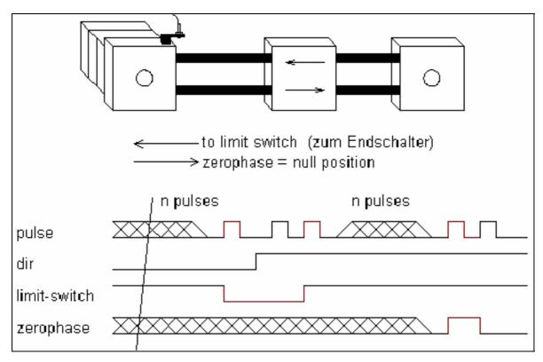
ZERO phase or ZERO position can be used as an exact reference point. Following is a procedure to handle with ZERO points.
