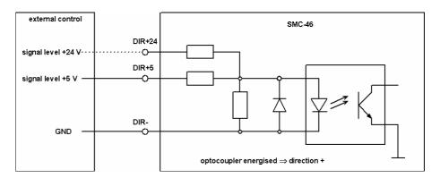
The Direction input determines the direction of motor rotation. There must be a pause of at least 120 µs between the time at which the direction of rotation is changed and enabling of the Clock input.
