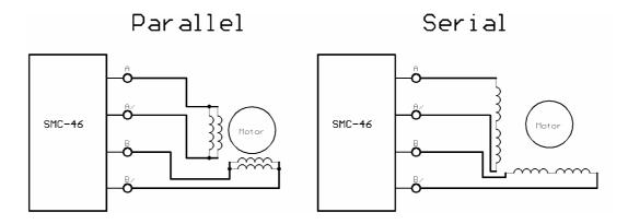
Refer to the data sheet of your stepper motor for the designations of your connecting cables. Check the connections carefully since a wrong connection can result in the output stage being destroyed.
