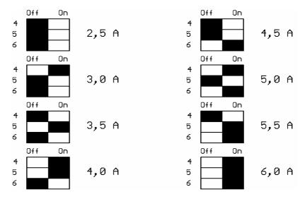
The set phase current is applied following power-up or after a reset (via pushbutton).
