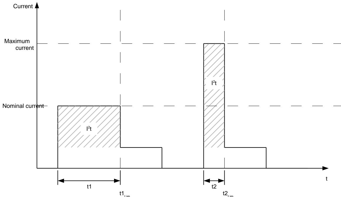
In the first section  $t_1$ , the current value is higher than the nominal current. At time  $t_{1\text{Lim}}$ ,  $I^2t_{\text{Lim}}$  is reached and the current is limited to the nominal current. During the following time period  $t_2$ , a current comes that corresponds to the maximum current. Accordingly, the value for  $I^2t_{\text{Lim}}$  is reached faster than in time period  $t_1$ .
