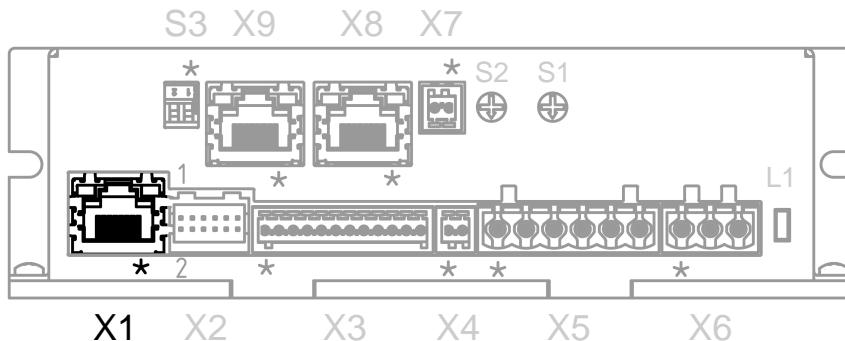
When communication occurs and data packets are received or sent, the yellow LED on the socket flashes.
