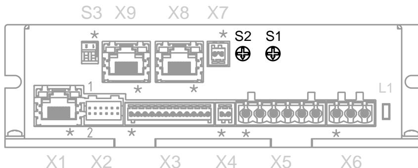
The following applies: S1 is the higher-value byte, while S2 is the lower value byte.
