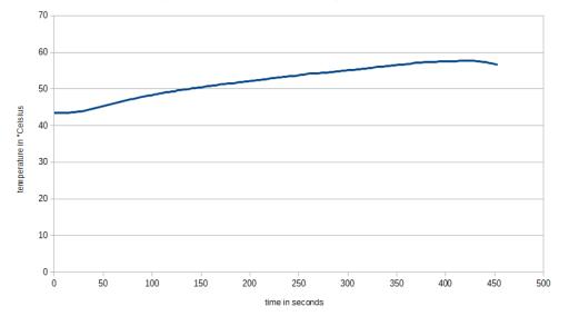
N5: Controller temperature at 45° Celsius ambient temperature and 18A motor current
