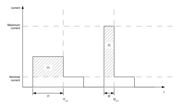
In the first section, t1, the current value is higher than the rated current. At time  $t1_{Lim}$ ,  $I^2t_{Lim}$  is reached and the current is limited to the rated current. A current that corresponds to the maximum current then occurs for a period of time t2. Hence, the value for  $I^2t_{Lim}$  is reached more quickly than in time t1.
