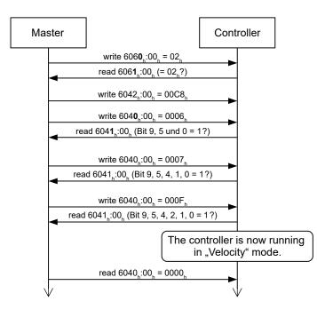
**4.** To stop the motor, set controlword  $(\underline{6040}_{h})$  to "6".
