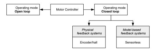
Summarized in the following are all possible combinations of control modes and feedback systems with respect to the motor technology. Support of the respective control mode and feedback is controller-specific and is described in chapters <u>Pin assignment</u> and <u>Operating modes</u>.
