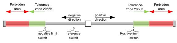
The previous figure shows the breakdown of the tolerance bands next to the limit switches:
