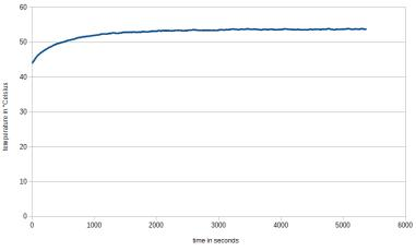
N5: Controller temperature at 45° Celsius ambient temperature and 18A motor current 70 60 50 temperature in "Celsius 40 30 20 10 0 ò 50 100 150 200 250 300 350 400 450 500 time in seconds
