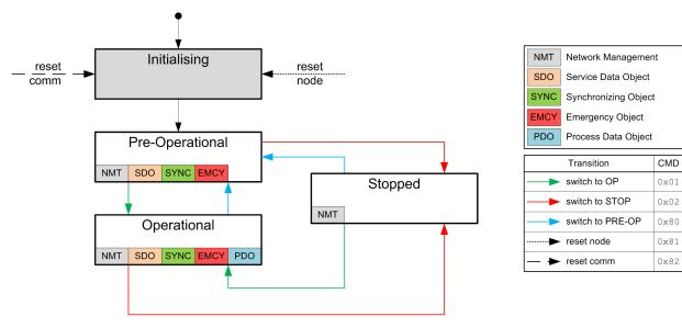
Shown in the following table is an overview of the activity of the services in the respective states. Note that the *Stopped* state stops communication completely and only permits controller of the NMT state machine.
