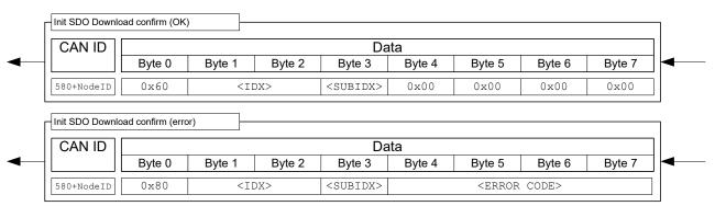
**Example**: Set object **607A**<sub>h</sub>:00<sub>h</sub> (target position, SIGNED32) to value  $3 \ge 8_h$  (=1000<sub>d</sub>) of a controller with node-ID 3:
