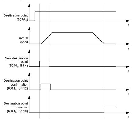
The controller can also reset bit 4 in object  $6040_h$  (controlword) on its own. This is set with bits 4 and 5 of object  $60F2_h$ .
