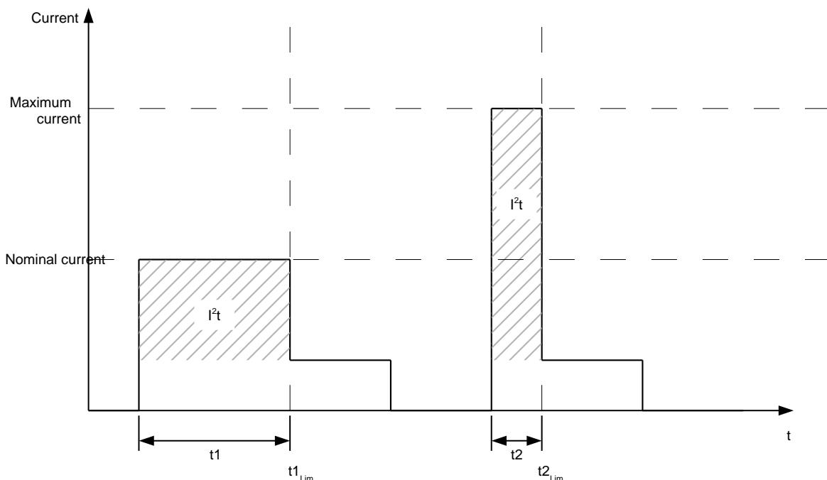
In the first section t1, the current value is higher than the nominal current. At time t1<sub>Lim</sub>, I<sup>2</sup>t<sub>Lim</sub> is reached and the current is limited to the nominal current. During the following time period t2, a current comes that corresponds to the maximum current. Accordingly, the value for I<sup>2</sup>t<sub>Lim</sub> is reached faster than in time period t1.
