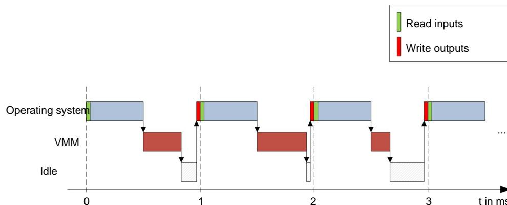
If the system detects that the user program requires more than the time assigned to it, it is closed and an error code is entered in the object directory. When developing user programs, therefore, the runtime behavior of the program must be carefully checked, especially in the case of time-intensive tasks. Therefore, it is advisable to use tables, instead of calculating a sinus value from a `sin` function.
