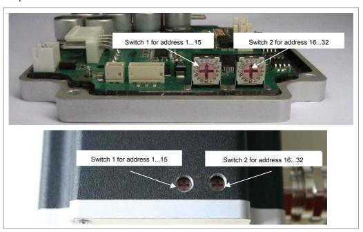
The 1st digit is set with switch 1 (left), the 16th digit of the address is set with switch 2 (right).
