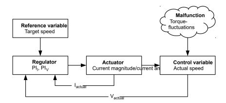
$PI_{l}$  = Proportional-integral current control loop  $PI_{l}$  = Proportional-integral velocity control loop
