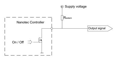
With a supply voltage of +24 V, a resistance value  $R_{external}$  of 10 k $\Omega$  is recommended.
