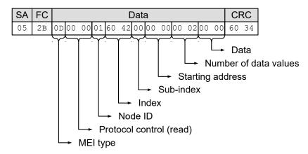
Shown as an additional example below, a sequence of Modbus messages is sent from the master to the slave to rotate the motor in "Velocity" mode:
