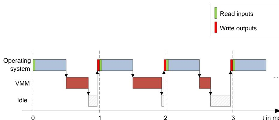
If the system detects that the user program requires more than the time assigned to it, it is closed and an error code is entered in the object directory. When developing user programs, therefore, the runtime behavior of the program must be carefully checked, especially in the case of time-intensive tasks. Therefore, it is advisable to use tables, instead of calculating a sinus value from a `sin` function.
