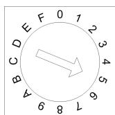
The NodeID can either be applied as a value from the adjuster wheel or read from object **2009<sub>h</sub>**.
