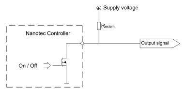
With a supply voltage of +24 V, a resistance value  $R_{external}$  of 10 k $\Omega$  is recommended.
