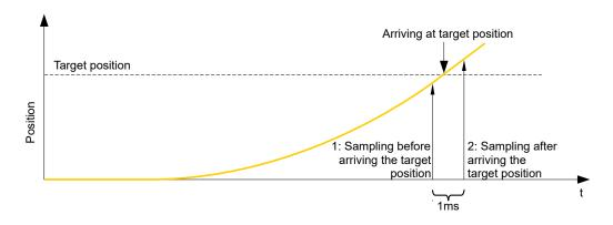
The current position is sampled once per millisecond. It is possible that the target position is reached between two samples. If the final speed is not equal to zero, then, after the target position is reached, the sample is used as an offset as the basis for the subsequent movement. As a result, the subsequent movement may go somewhat farther than expected.
