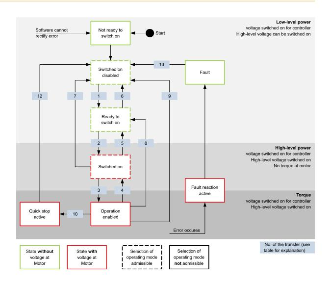
Listed in the following table are the bit combinations for the controlword that result in the corresponding state transitions. An X here corresponds to a bit state that requires no further consideration. The only exception is the resetting of the error (fault reset): the transition is only requested by the rising edge of the bit.
