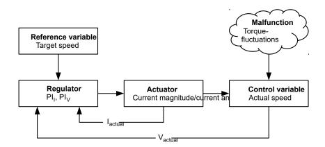
PI<sub>I</sub> = Proportional-integral current control loop PI<sub>V</sub> = Proportional-integral velocity control loop
