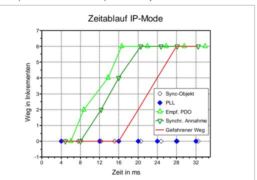
The following figure shows the time progression in Interpolated Position mode. The time is plotted on the x-axis and the position on the y-axis.
