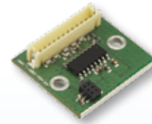
Magnetic encoder, customized for integration
